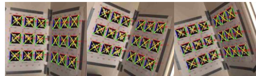
Figure 3 Intrinsic calibration of camera
